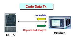
The option can verify the network response when DUT receives correct data and also wrong data by using transmission function that can combine maximum 256 code data and Auto-Negotiation analysis function.
