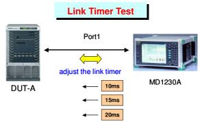
The option can confirm DUT performance by changing Link Timer value. Variable range is from 0ms to 100ms that make more extensive performance test than standard.
